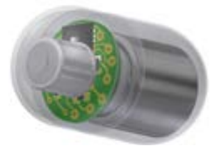
Illustration of a swallowable capsule with built-in gas sensor, microprocessor and wireless high-frequency transmitter. Image: Nam Ha.
