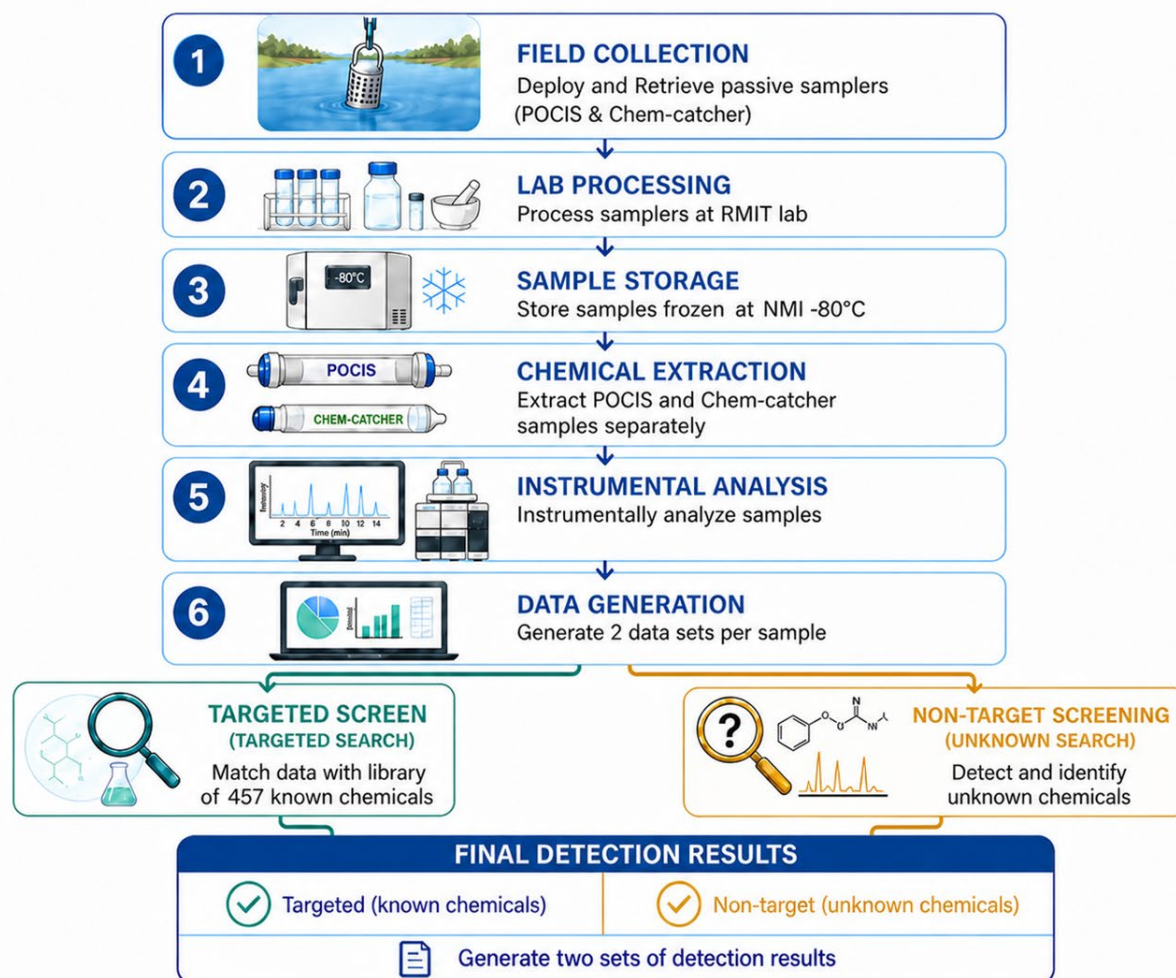
Figure 1 Workflow overview of passive sampler processing for the Polar Organic Chemical Integrative Sampler (POCIS) and Chem-catcher, High Resolution Mass Spectroscopy (HRMS) analysis, and data generation leading to targeted and non-target screening outputs.
