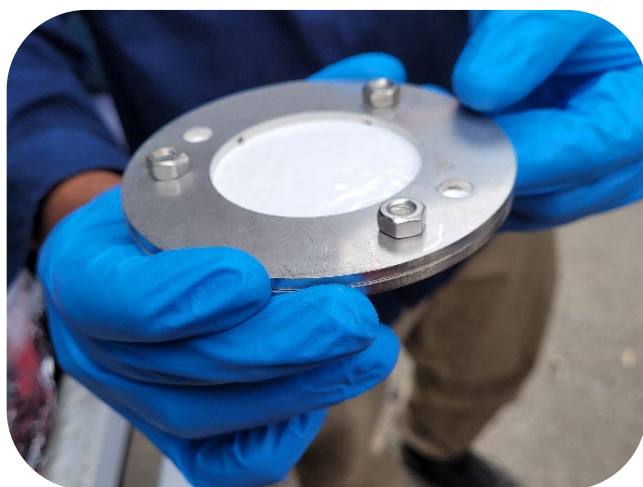
POCIS passive sampler and its housing (left) and Chemcatcher sampler and its housing (right).
