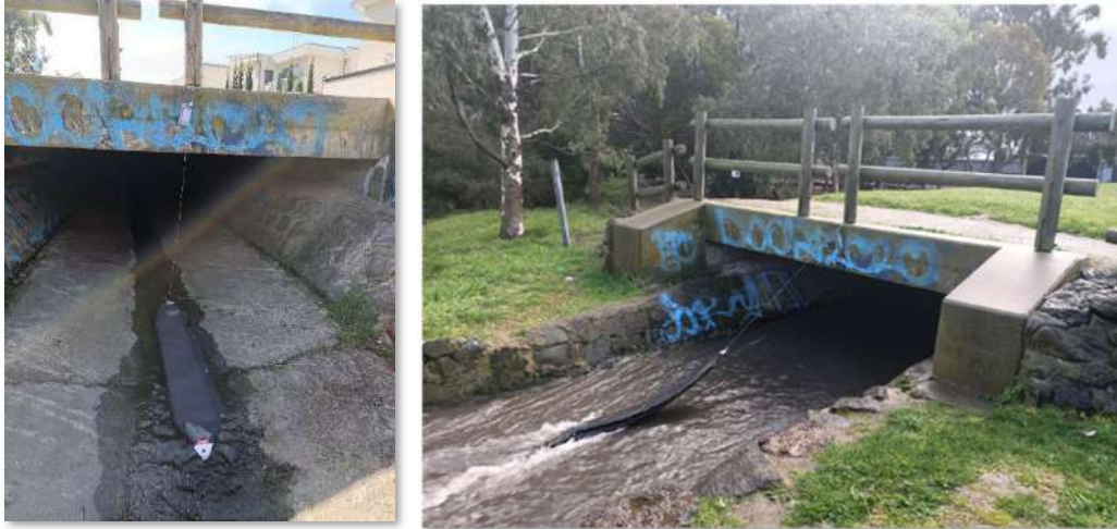
Figure 4. Sediment bag deployed in Graingers Rd Main Drain (Charlotte St). Sediment bags are tethered to structures in stormwater drains using wire cables and trap sediment particles from stormwater.
