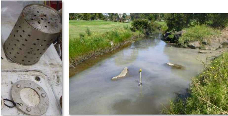
Figure 2. Polar Organic Chemical Integrative Sampler (POCIS) passive sampler and stainless steel cage. Passive samplers are used to measure water soluble contaminants, and are deployed instream, attached to a steel picket.
