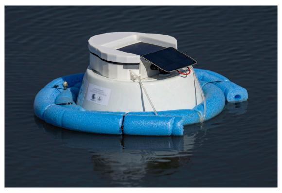
**Fig. 3:** Photo of a Pondi – one of CNPS' floating greenhouse gas sensors equipped with CO<sub>2</sub>, CH<sub>4</sub>, and N<sub>2</sub>O sensors to continuously measure gas concentrations within the chamber. All data is sent to a cloud via 4G, allowing for the real-time monitor of greenhouse gas fluxes. Each Pondi is equipped with a solar panel for continuous battery charging and a robotic pump (white U-shaped structure) for periodic venting to prevent gas saturation within the chamber.
