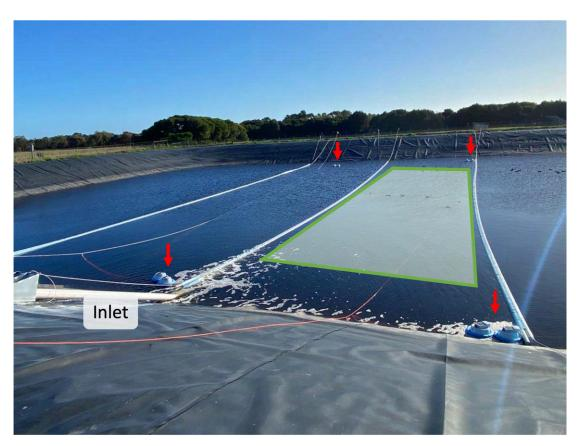
**Fig. 4:** Baseline monitoring using Pondi (marked by red arrows) deployed within the treatment (on the right-hand side of the lagoon inlet) and control (on the left) channels. The shaded green area indicates the deployment location of the CFW.
