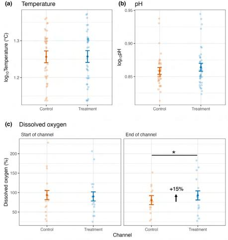
**Fig. 12:** Average (a) temperature (in °C), (b) dissolved oxygen concentrations (in %), and (c) pH in the control (orange) and treatment (blue) channels across the sampling period. Error bars indicate standard errors.
