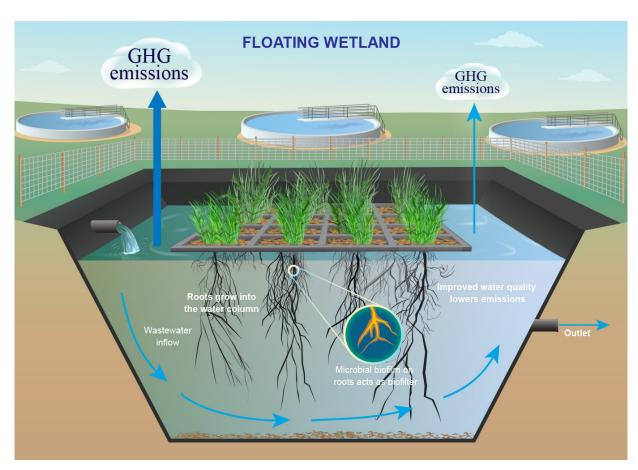
**Fig. 1:** Schematic of a constructed floating wetland (CFW) that was deployed at the Westernport WWTP storage lagoon. With roots growing into the water column, wetland plants can take up nutrients from the water, which is expected to result in a reduction in greenhouse gas emissions from the lagoon.
