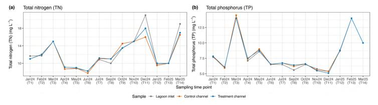
**Fig. 8:** (a) Total nitrogen and (b) total phosphorus (in mg <sup>L-1</sup>) at the lagoon inlet (grey) and at the end of the control (orange) and treatment (blue) channels.
