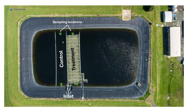
**Fig. 2:** Storage lagoon with the control and treatment (floating wetland) channels. The inlet to the lagoon is connected to a splitter box that allows for equal water inflow into the two channels. Stars indicate the four sampling locations (i.e., start and end of the control channel, start and end of the treatment channel) for greenhouse gas fluxes, dissolved nutrient levels, and water quality parameters.
