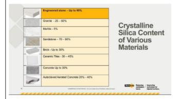
When these materials are worked on, silica is released as a fine dust known as respirable crystalline silica or silica dust.
