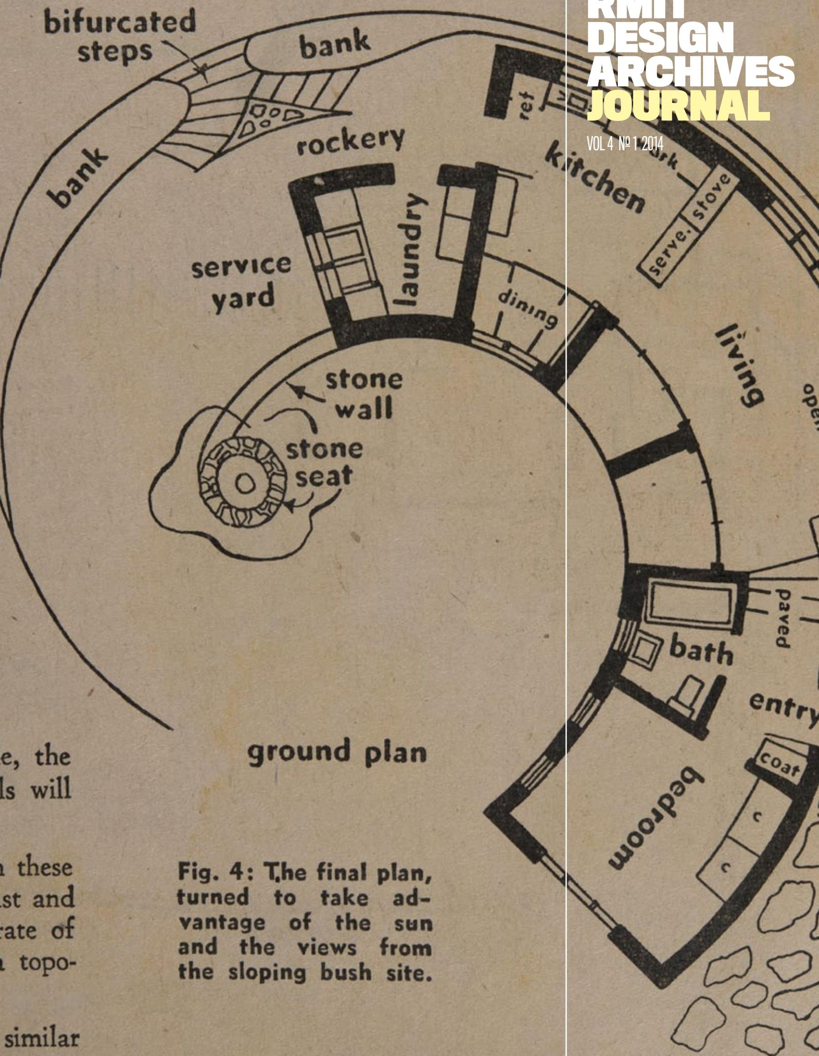
**Fig. 4: The final plan, turned to take advantage of the sun and the views from the sloping bush site.**
