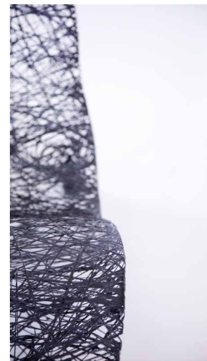
Random Chaise , designed by Kitty Cao, is an airy, lightweight furniture art piece. It was made by wrapping 12,000 carbon fibre strings around a mould while squeezing epoxy resin into the strings.
