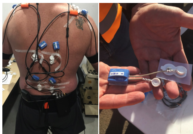
FIGURE 2: The wearable sensor system. REFERENCE(S): 3.0, p. 61.
