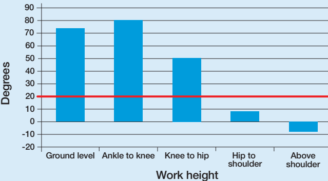
FIGURE 6: Average back (trunk) inclination (bending) when using pincer cutting tool to tie steel reinforcement bars by work height. REFERENCE(S): 4.1, p. 86.
