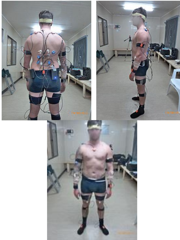
Figure 3.4: Sensor placement shown on one participant's front, side and back. Xsens sensors are orange. EMG sensors are blue.
