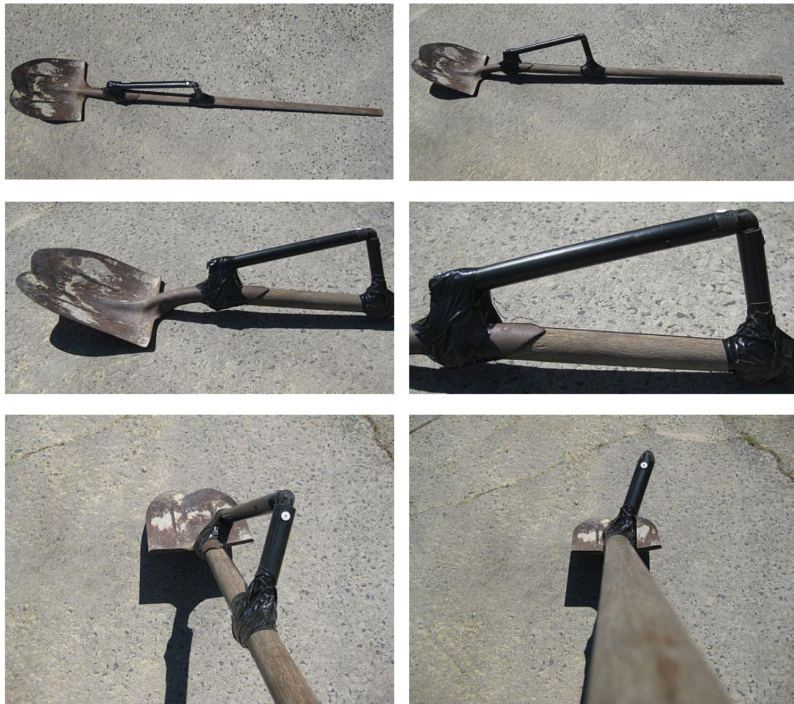
Figure 8.3: Images of range of views of supplementary handle design on long handle shovel.
