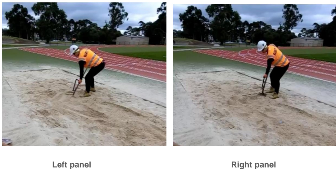
Figure 8.4: Participant 12 using usual handle (left panel) and supplementary handle (right panel) for shovelling.
