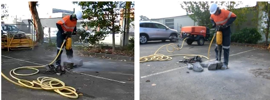
Figure 7.1: Assessment equipment test at site 1 – jackhammering demonstration using bluestone blocks.
