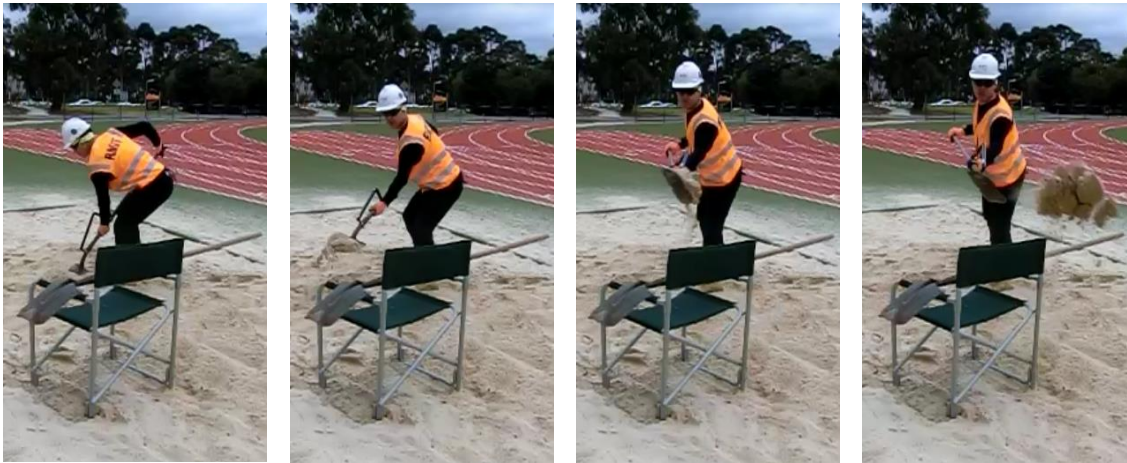
Figure 8.5: Participant 11 shovelling sand over a barrier to imitate loading a wheelbarrow.
