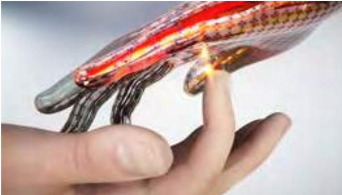
*The prototype device developed by a team at RMIT University can electronically replicate the way human skin senses pain.*
