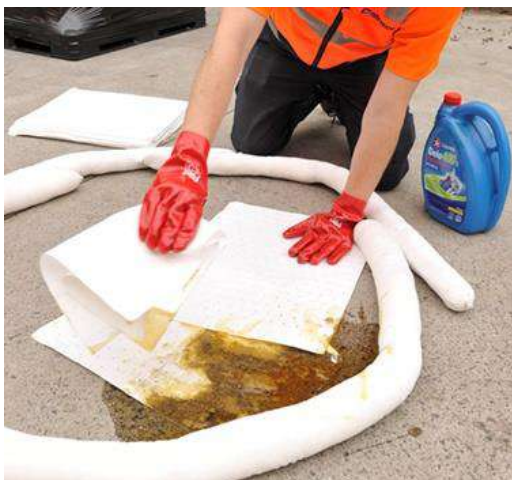
Figure 7.4. Containment and cleanup of a spill.
