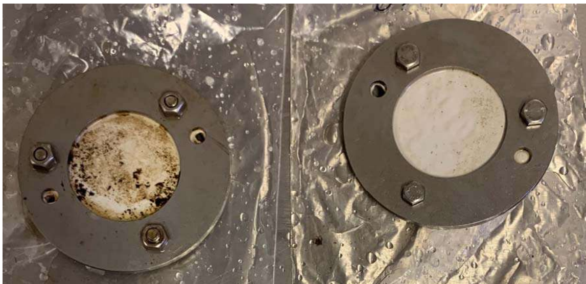
Plate 6: POCIS passive samplers following retrieval
