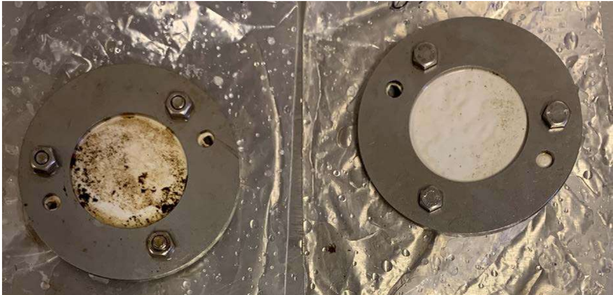
Plate 6: POCIS passive samplers following retrieval.
